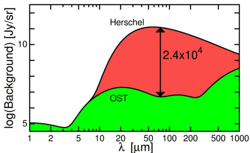
The low detector background due to using a cold telescope and the larger aperture make OST  $>1000x$  more sensitive than Herschel.
