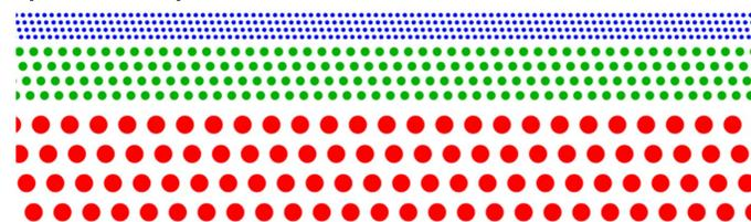
Possible focal plane arrangement for a three band fast scanning photometer.
