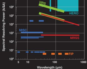
Leveraging improvements in detector technology and a large, cold primary mirror, OST will offer two to four order of magnitude improvement in sensitivity over Herschel. OST will bring arc-second imaging and unprecedented spectroscopic capabilities to the infrared universe.
