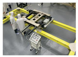
Figure 2-45: Variable Center of Gravity Mechanism
