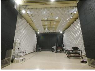
Figure C-73: Large EMC Shielded Enclosure
