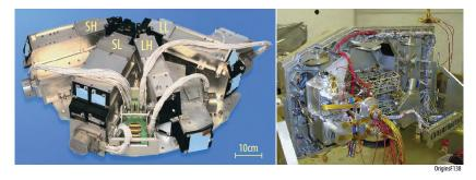
**Figure 3-11:** Previous missions provide heritage for the basic approach of the OSS elements. The bolted aluminum OSS grating spectrometer uses the same approach as the Spitzer infrared spectrograph from Houck et al., 2004. Its four wideband modules are shown at left. The Fourier-transform module path-folding approach and mechanism use the same approach as in the Herschel SPIRE instrument shown at right (Griffin et al., 2010).
