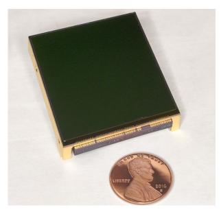
**Figure 3-24:** Long-wavelength HgCdTe detectors have been developed for NASA's NEOCam mission.
