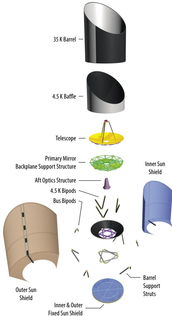
**Figure 2-15:** (left) *Origins* CPM components exploded view shows the *Origins* configuration. Instruments are not shown in this diagram.
