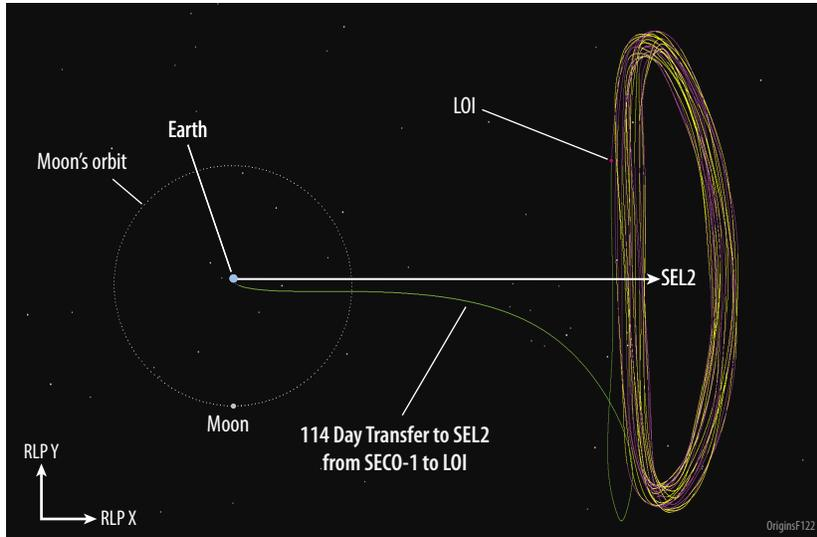
**Figure C-81:** *Origins* transfers to SEL2 over 114 days before executing a LOI maneuver to insert itself into the mission orbit.
