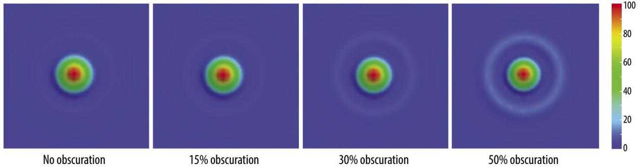
**Figure C-49:** Comparison of PSFs for increasing values of linear obscuration for an on-axis telescope
