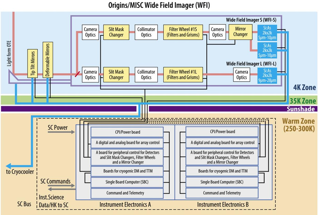
**Figure D-16:** The MISC WFI block diagram indicates the second module that was added to the upscoped MISC instrument.
