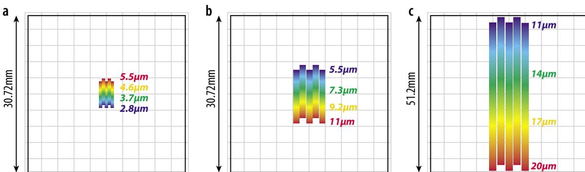
**Figure 3-18:** The spectra from the five pupil slices are overlaid on the short, mid, and long focal planes as shown in panels a-c, respectively.
