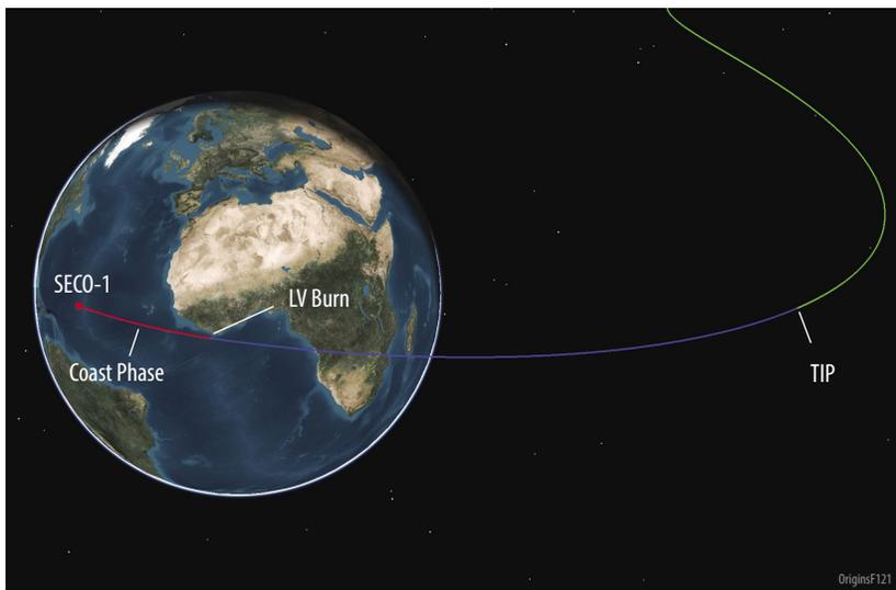
**Figure C-80:** *Origins* will then coast along its parking orbit until a state is reached where the Launch Vehicle will perform a large maneuver that will place *Origins* on the correct outbound trajectory to SEL2.
