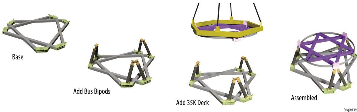
**Figure C-16:** The Bus Bipods are temporarily supported during assembly since they are hinged at the base.
