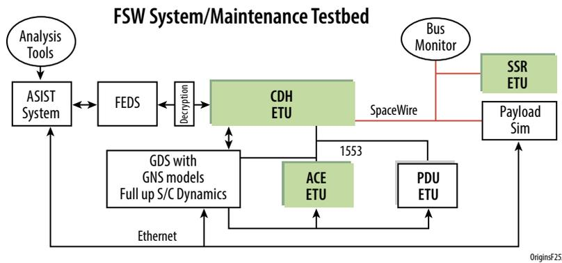
**Figure C-64:** Flight Software System Test Environment
