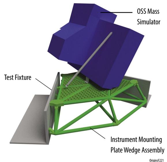
**Figure C-40:** Telescope Wedge ETU Test Setup is inverted during ground-testing, which allows less-robust ground support equipment to support the unit during the tests.
