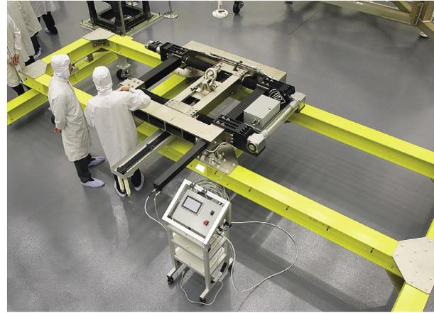
**Figure 2-45:** Variable Center of Gravity Mechanism
