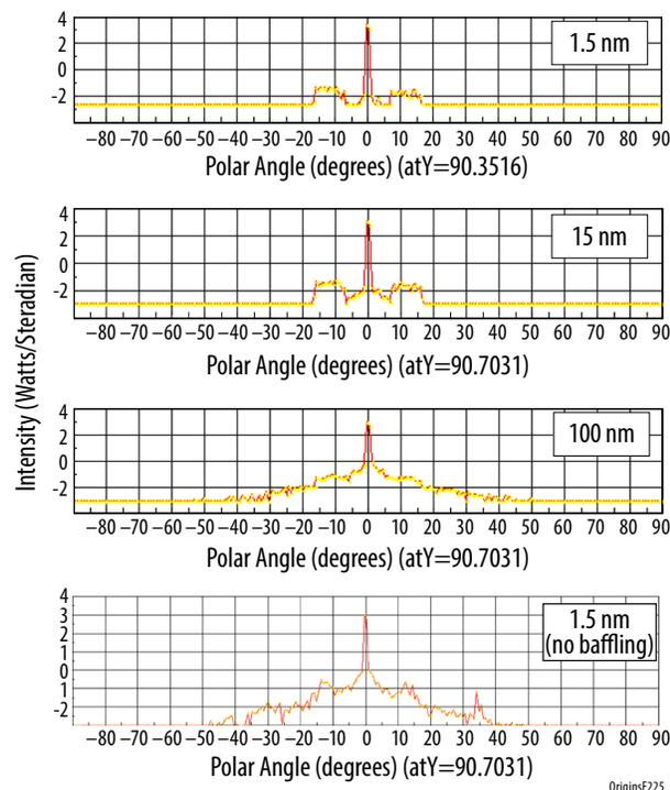
**Figure C-43:** (Above) Analysis showing relative intensity between the desired signal (the instruments' FOV footprints) and noise due to near field scatter. Note that the x and y lines scans are plotted on a logarithmic scale and show between about four and five orders of magnitude difference between signal and noise. Calculations carried out at  $\lambda = 30\mu\text{m}$ .
