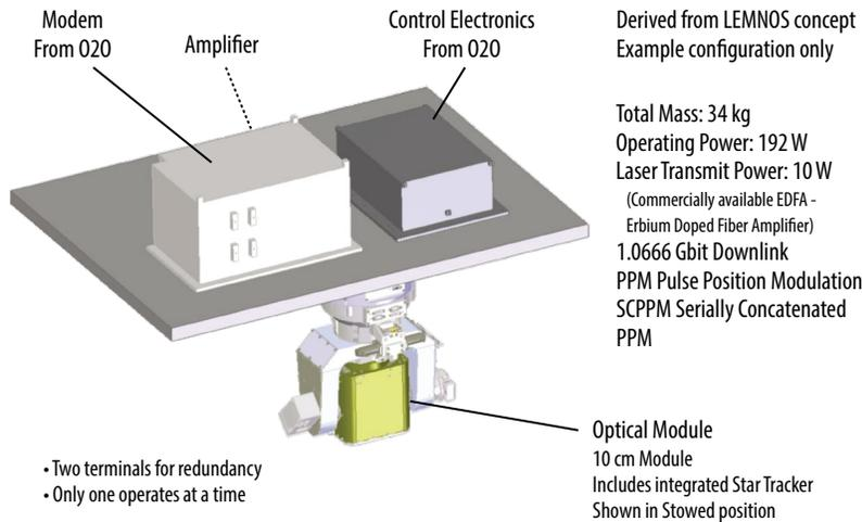
**Figure 2-39:** The *Origins* optical communication system is fully redundant.
