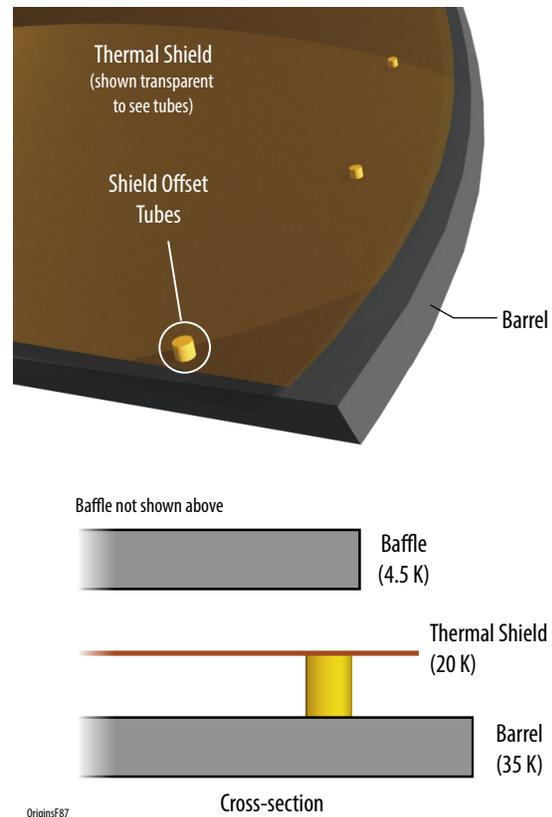
**Figure 2-19:** The Thermal Shield is offset from the Barrel to provide an effective radiative shield. The shield is fastened to thin-walled Vespel® tubes mounted to the inside of the Barrel.
