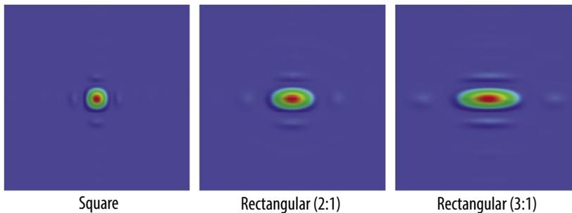
**Figure C-51:** PSFs for square and rectangular aperture shapes. Such apertures were deemed unacceptable for *Origins* due to yielding an asymmetric PSF.
