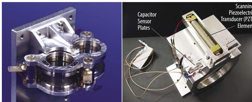
**Figure 3-12:** Heritage of scanning etalons for far-IR astrophysics. Left shows the dual etalon used in the Infrared Space Observatory (ISO) (credit Max Planck Institute for Extraterrestrial Physics, Garching).
