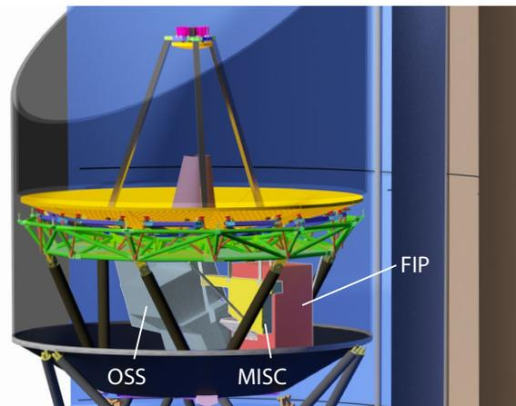
**Figure 2-32:** Each instrument under the backplane of the primary mirror assembly. This location is effective for maintaining the instruments (and mirror) at 4.5 K in the cryo-payload module (CPM, Section 2.3).
