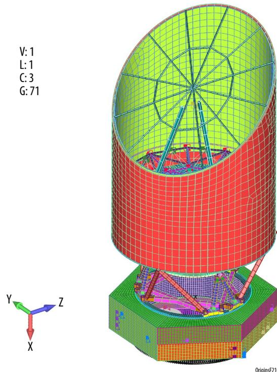
**Figure C-29:** The *Origins* observatory finite element model shows a very detailed design for an accurate first-cut analysis. Colors denote different components.
