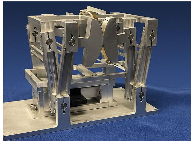
**Figure 3-7:** Flex type mechanism for use with the OSS FTS. This mechanism is free of friction, can be operated in any orientation and has a stroke of 10 mm. For OSS this would be scaled up by a factor of 3.
