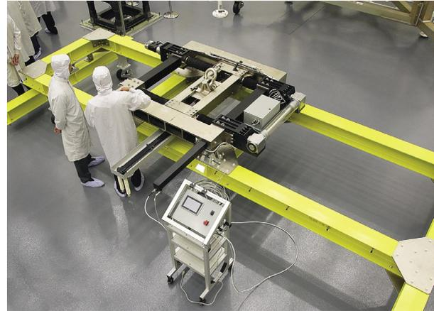
**Figure 2-45:** Variable Center of Gravity Mechanism
