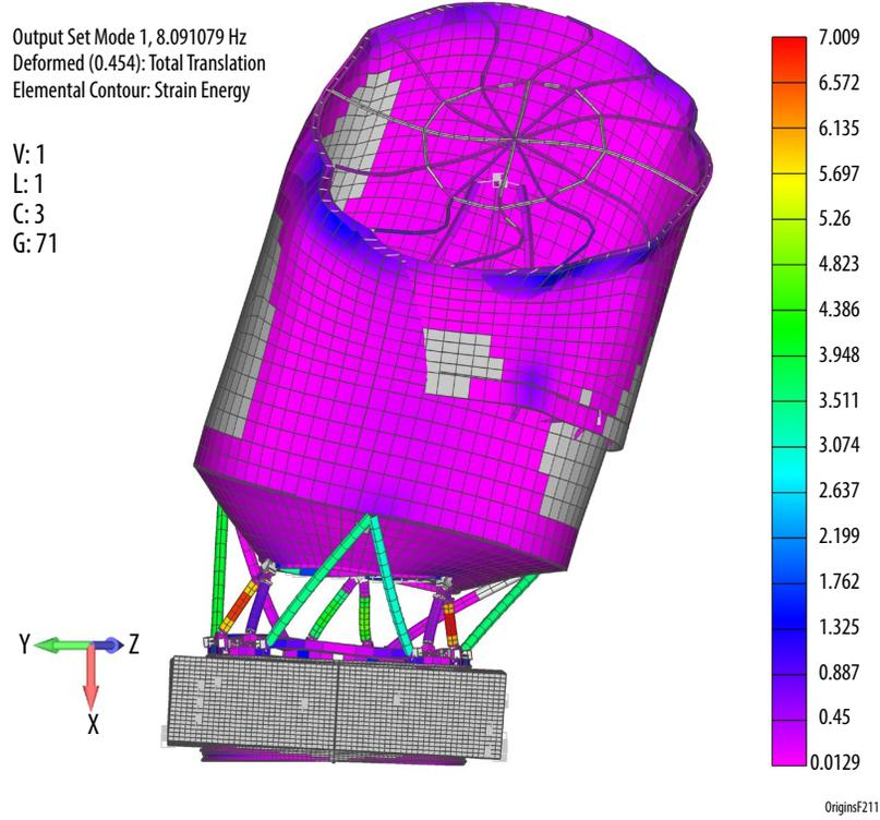
**Figure C-30:** Primary lateral frequency mode shape is driven by the barrel of the observatory. Colors denote strain energy levels.
