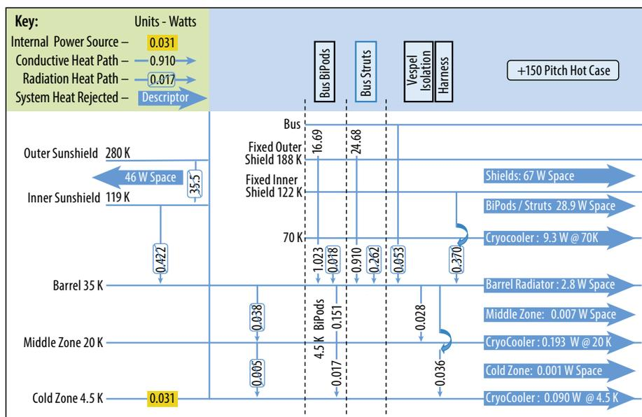
**Figure 2-8:** *Origins* Heat Flow Map of the CPM shows the multiple stages of cooling results in a reasonably small heat load to the cryocooler and radiative cooler stages
