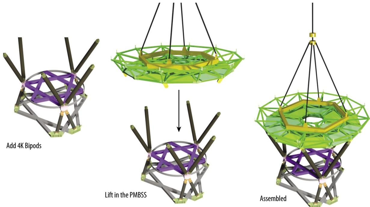
**Figure C-17:** The 4.5 K Bipods are supported until the PMBSS is installed.
