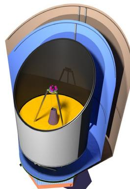
**Figure 2-14:** (below) The *Origins* on-orbit configuration, with the sunshields deployed, is ~13 m long and ~9 m in diameter
