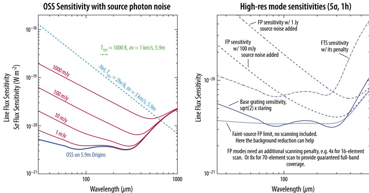
**Figure 3-10:** Sensitivity of OSS for bright sources (left) and in the high-resolution modes (right). The etalon (FP) curves refer to the required scanning time to be incorporated
