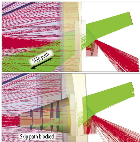
**Figure C-41:** (Above) External (left) and internal (right) baffles. Both sets of baffling are meant to stop the ability of unwanted light sources from reaching the focal surface.
