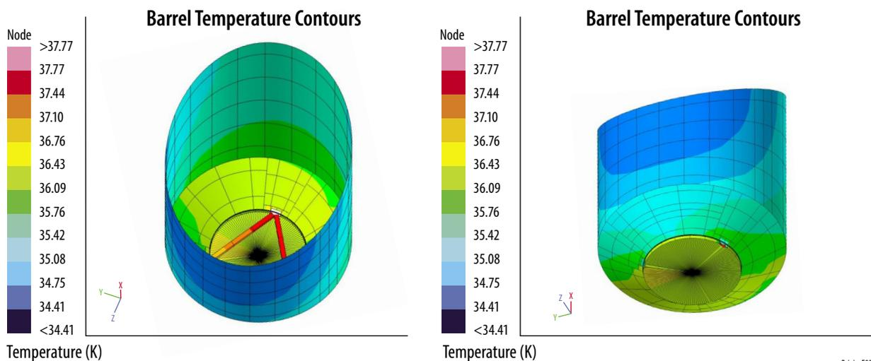
**Figure 2-12:** The Barrel temperature contours show that the barrel temperature remains below 36 K and nearly isothermal in the worst case attitude (150° pitch) over nearly all of its surface.
