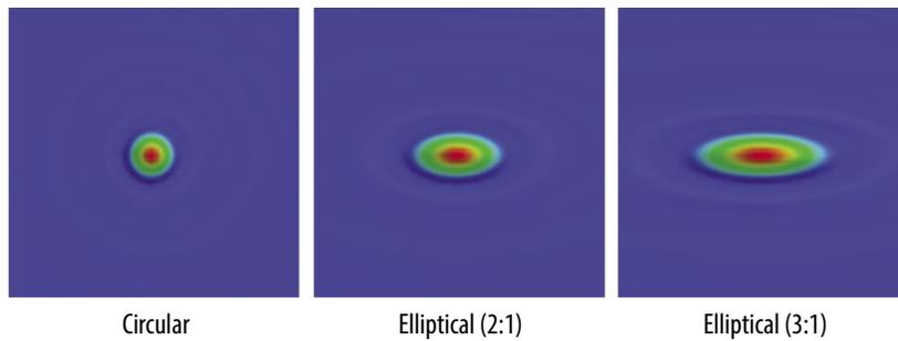
**Figure C-50:** PSFs for circular and elliptical aperture shapes showing that asymmetry in the aperture shape leads to undesired asymmetry in the PSF. The circular aperture was chosen for *Origins*.
