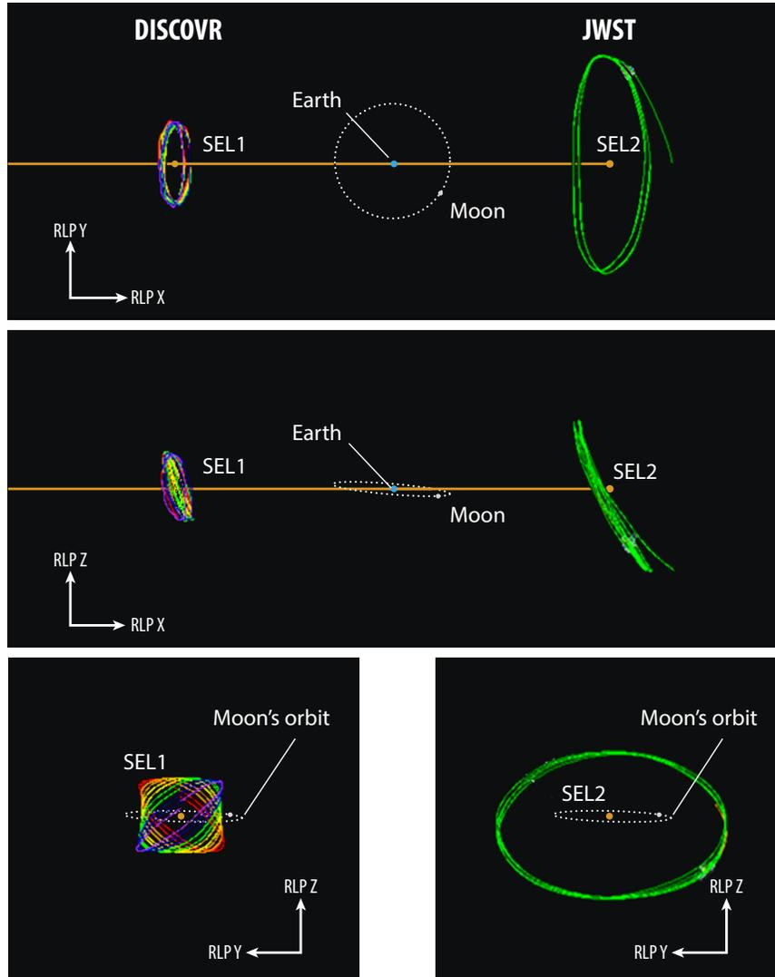
**Figure C-77:** JWST and DSCOVR orbits are shown in the XY, XZ, and YZ Rotating Libration Point Frame show examples of the various orbits (shown to scale) that can be achieved at the Libration Points.
