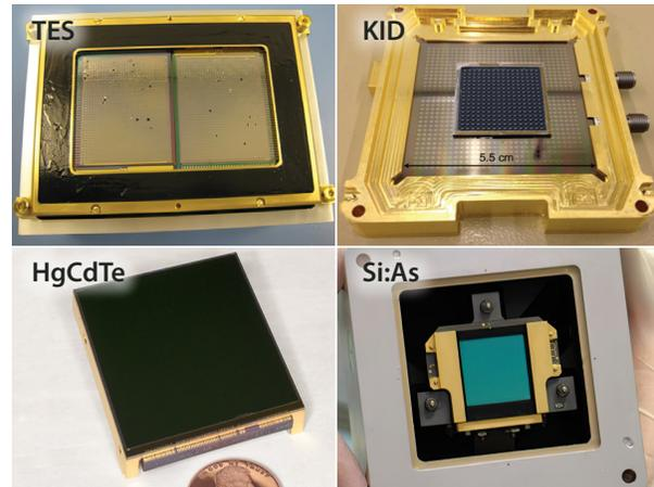
**Figure ES-10:** The robust *Origins* Technology Development Plan recommends parallel investment in four detector technologies. TES bolometers (HAWC+ array), KIDS (432-pixel device), HgCdTe arrays (JWST/NIRCam), and Si:As (JWST/MIRI).
