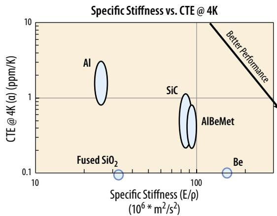
**Figure C-53:** The coefficient of thermal expansion (CTE) at 4.5 K plotted against specific stiffness at room temperature shows beryllium (Be) is the best performer, followed by AlBeMet®, SiC, fused silica, and aluminum (Al).
