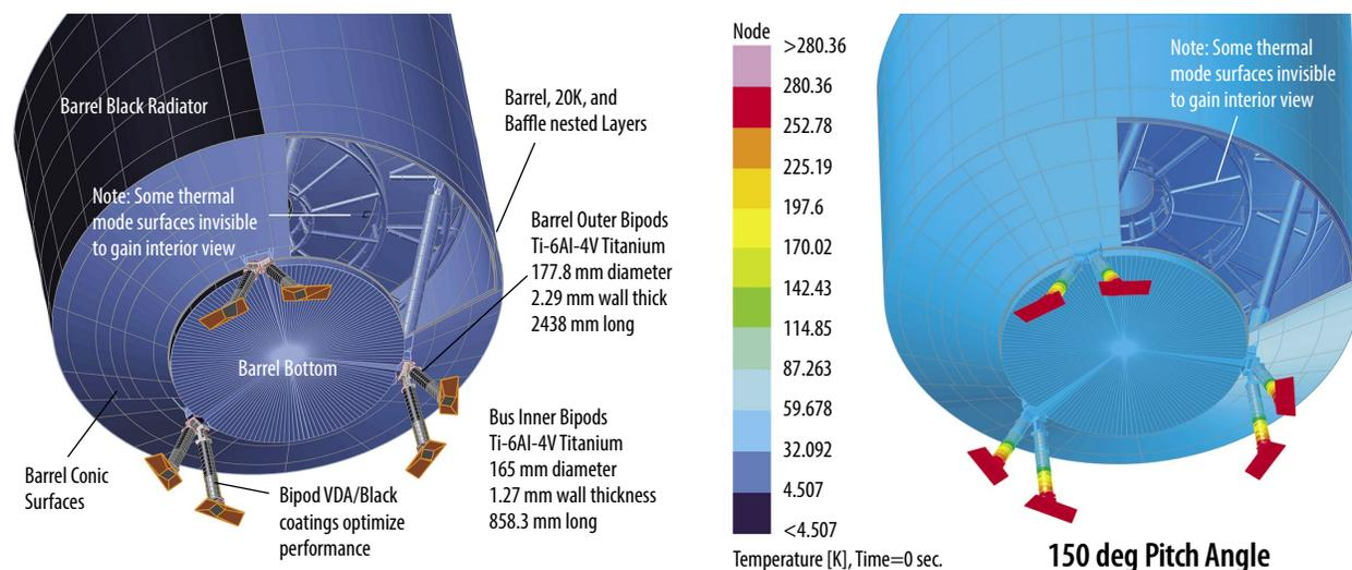
**Figure C-5:** The thermal model shows that the Bus bi-pods effectively thermally isolates the CPM from warmer SBM.
