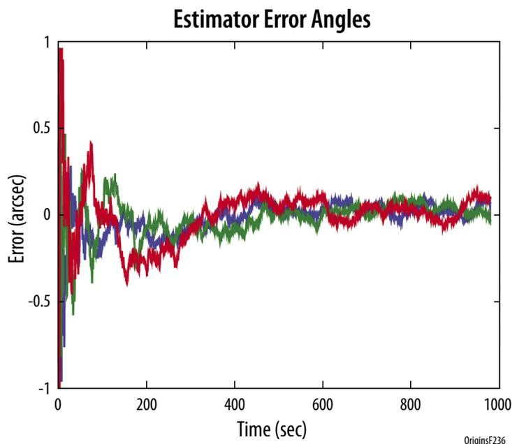
**Figure C-57:** Pointing knowledge during inertial hold is validated by time-domain simulation. Although the Kalman filter requires several minutes to achieve steady-state performance, pointing knowledge is within the 150-mas RMS requirement after only 10 seconds of initialization.
