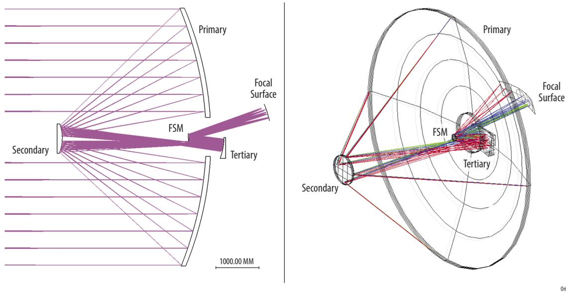
**Figure 2-22:** *Origins* baseline telescope layout shows the locations of the four mirrors and focal surface from both side (left) and perspective (right) views.
