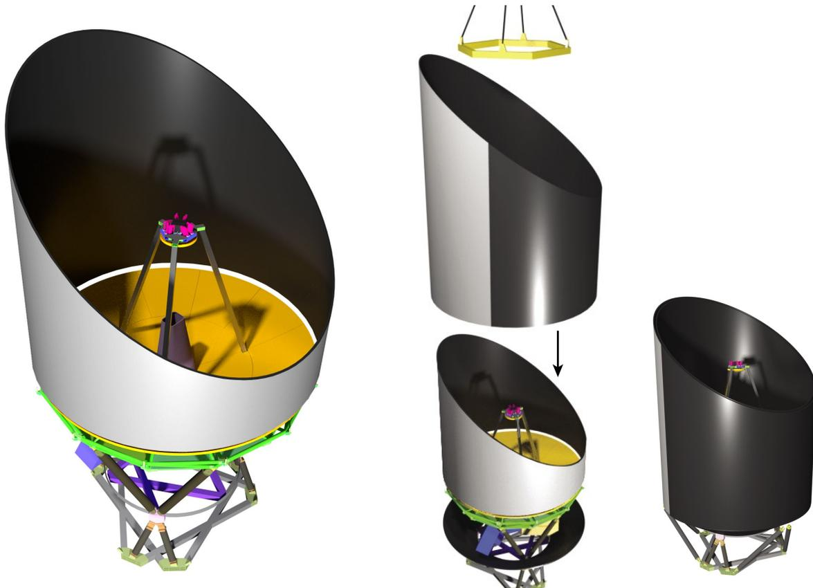
**Figure C-20:** Titanium flexures are installed on the PMBSS, located around the entire top edge of the PMBSS, and then the Baffle is lowered down and attached to the flexures.
