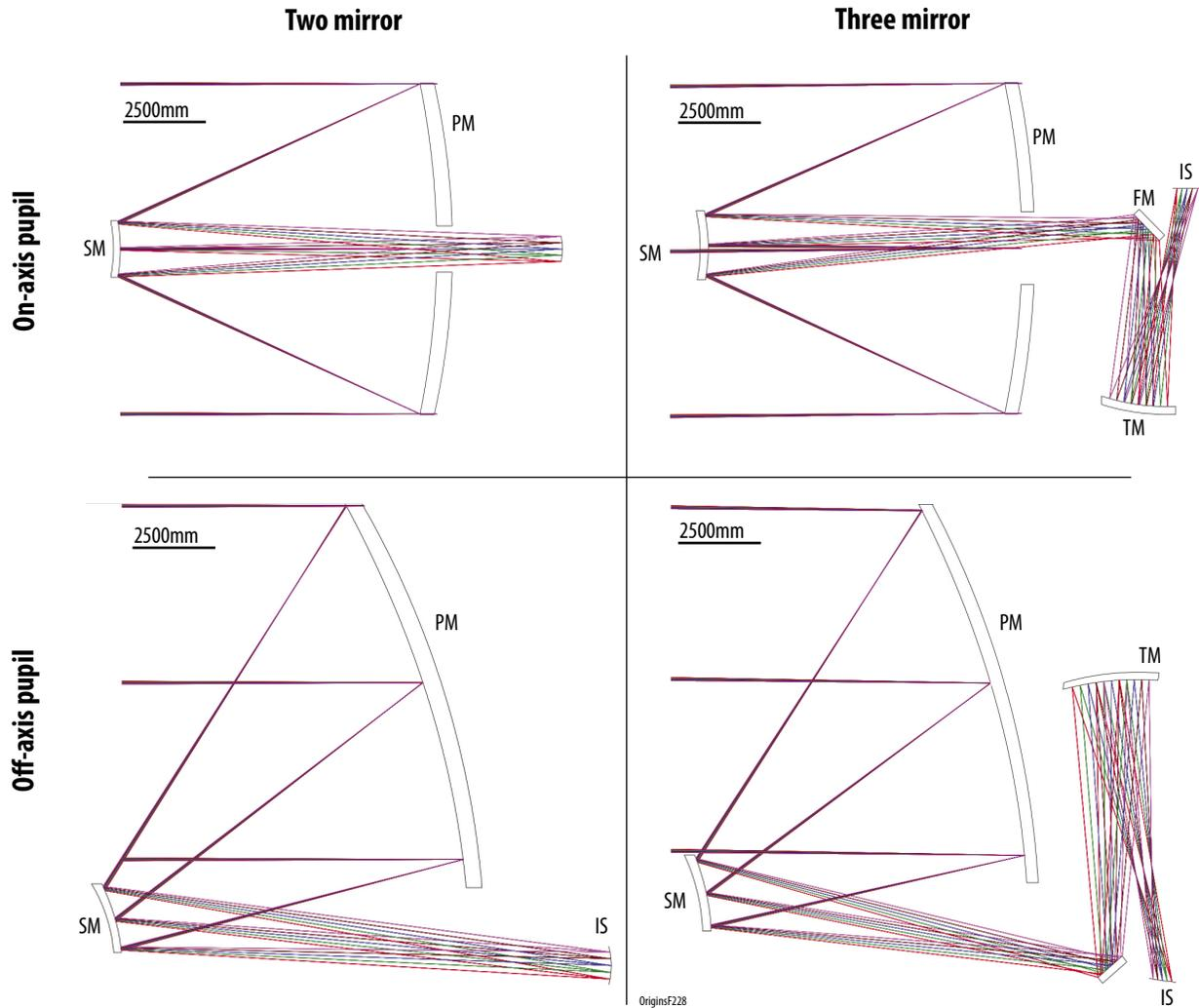
**Figure C-47:** Comparison showing the different optical layouts for each of the four telescopes configurations identified for study. A variant of configuration C was chosen for *Origins*.
