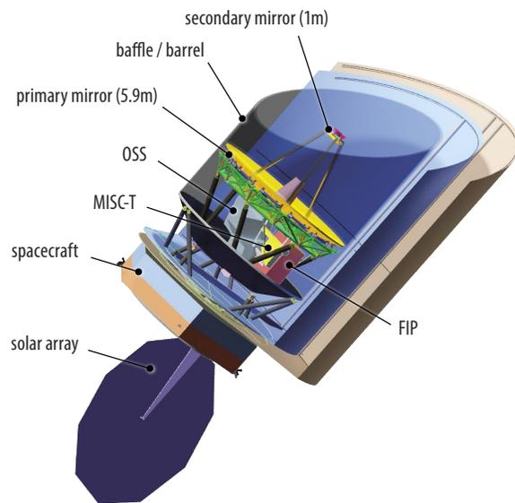
**Figure ES-8:** *Origins* builds on substantial heritage from *Spitzer* to minimize assembly, integration and testing, and deployment risks. A cutaway view shows the *Origins* instrument locations and major elements of the flight system.
