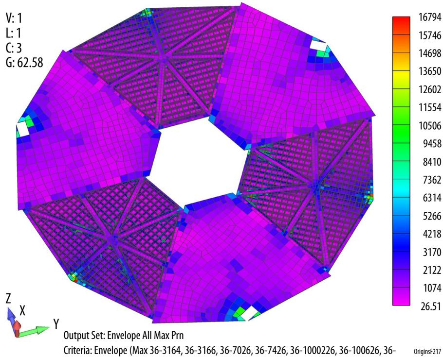
**Figure C-36:** The highest stressed beryllium plate component is along the outside edge of an IMP. Color denotes stress levels (PSI).
