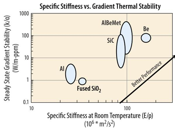
**Figure C-54:** Steady state gradient stability plotted against specific stiffness at room temperature shows beryllium (Be), AlBeMet®, and SiC as the best performers.
