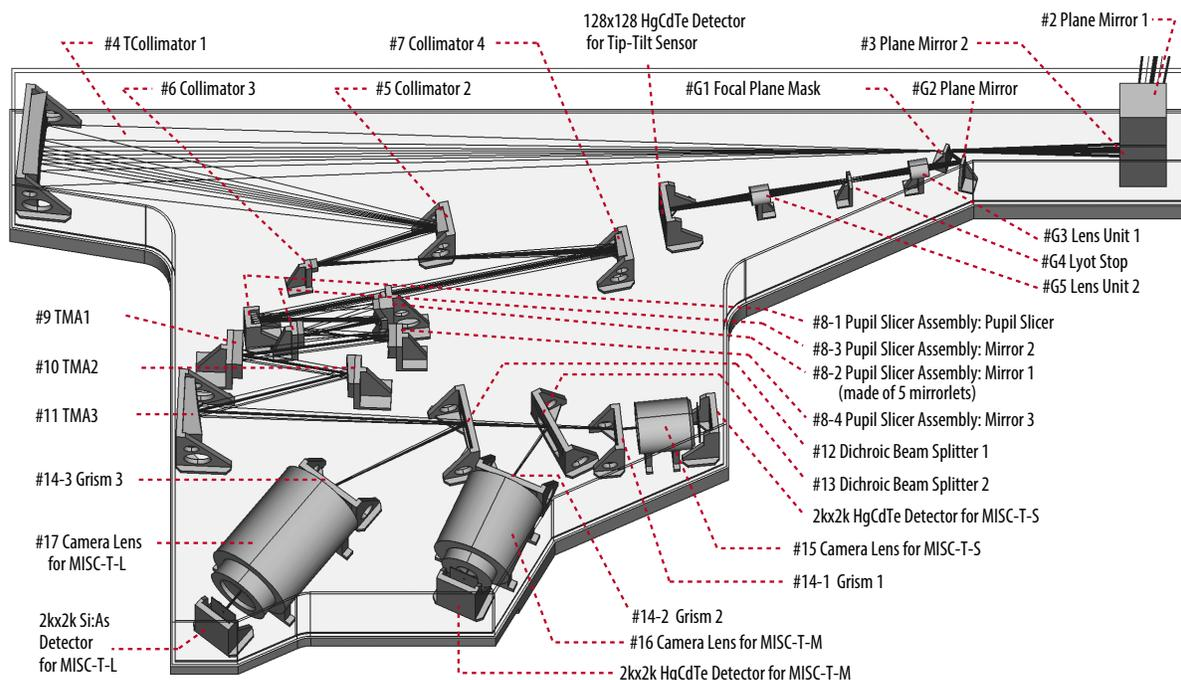
**Figure 3-20:** A 3D solid model of the MISC-T instrument indicating the optical path of the light within the instrument and the location of the mechanical components on the optical baseplate.
