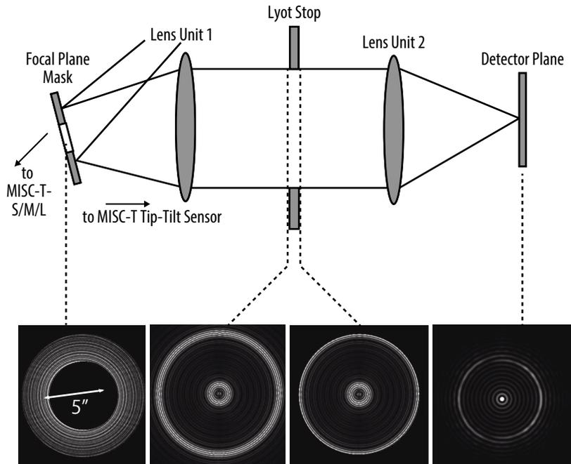
**Figure 3-19:** A schematic view of the MISC-T TTS showing the results of a simulation of a PSF image A) at the Lyot-Coronagraph focal plane mask, B) just before the Lyot stop, C) just after the Lyot stop, and D) at the detector plane.
