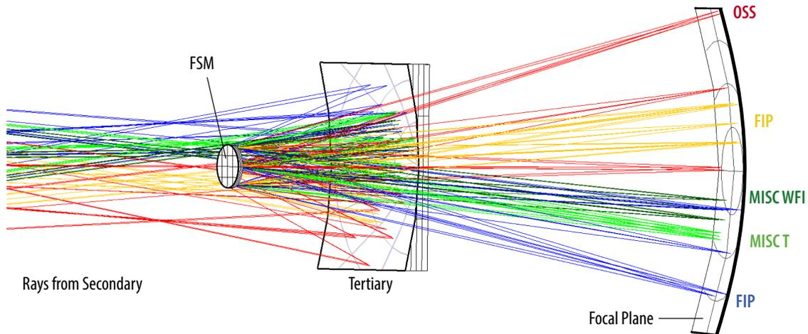
**Figure 2-26:** CODEV® layout showing rays for each of the three baseline instruments passing through the telescope onto the image surface.
