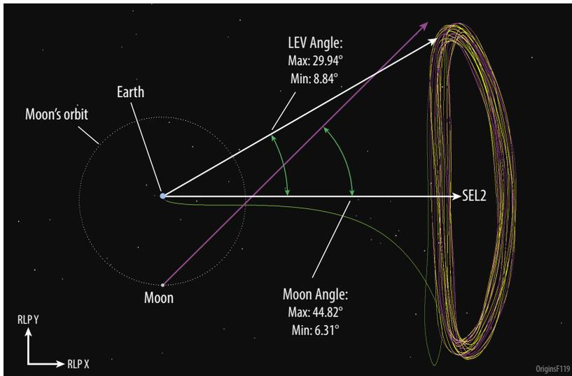
**Figure C-78:** *Origins'* transfer trajectory and mission orbit for 10 years shown in the RLP XY Frame with corresponding LEV and Moon Angles meets current requirements
