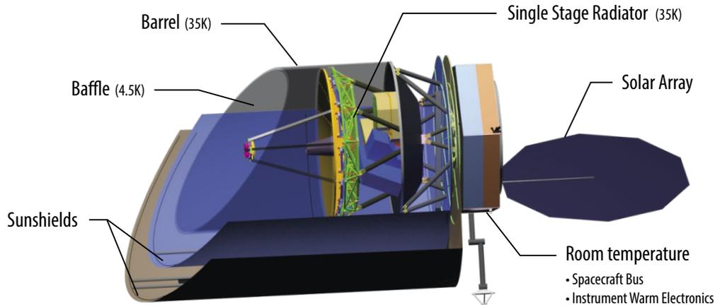
**Figure 2-5:** *Origins* temperature zones are designed to maximize cryo-cooling efficiency while ensuring a 4.5 K environment for the telescope and instruments. The instruments are housed in the 4.5 K zone beneath the primary mirror. The 35 K radiator is more clearly shown in Figure 2-9.
