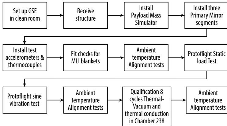
**Figure C-39:** The Telescope Wedge ETU Test Flow shows the rigorous testing performed to ensure good optical performance and robust tolerance to launch loads.
