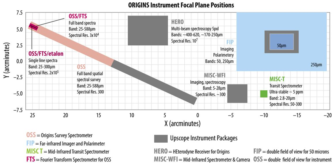
**Figure 2-2:** The *Origins* Space Telescope focal plane showing all the instruments studied and the result of the descope exercise. Those items shown in grey were descope and two (HERO & MISC-WFI) of these are described as possible upscoopes in Appendix D.
