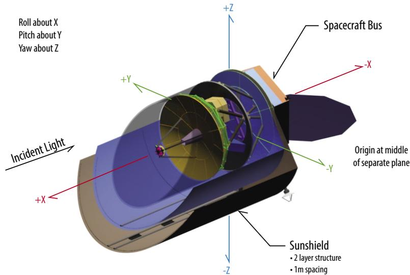
**Figure 2-7:** *Origins* cut-away view showing the observatory coordinate system. The Spacecraft Bus Module is toward the back right in this view and the Cryogenic Payload Module is everything front and left of that including the telescope barrel and sunshields. The *Origins* coordinate system uses +X as the boresight and -Z as the direction to the Sun when the pitch angle is 90 degrees and the roll is 0 degrees.
