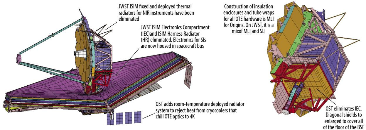
**Figure F-2:** View of the JWST derived *Origins* Alternate Architecture
