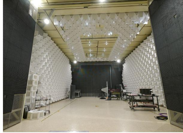
**Figure C-73:** Large EMC Shielded Enclosure
