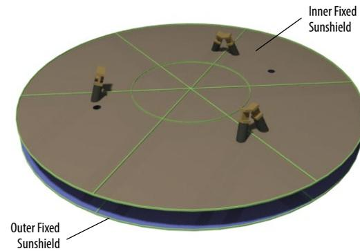
**Figure 2-21:** Fixed Sunshields are mounted along the Bus Bipods at the appropriate position to optimize thermal shielding. The deployed shields are attached to the respective Fixed Sunshield. Thermal closeouts are taped to the bipods and struts (Deployable shields not shown for clarity).
