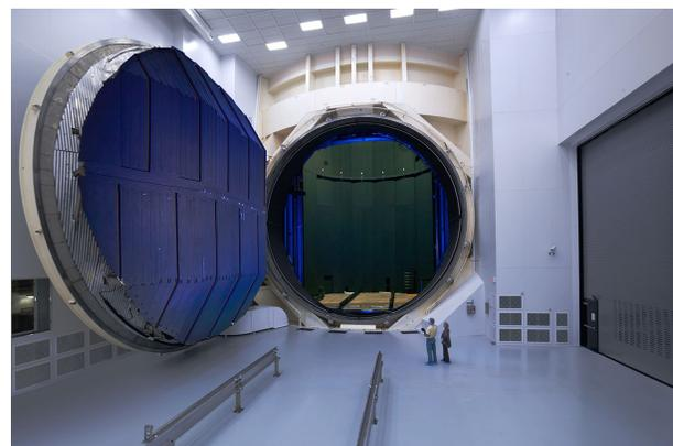
**Figure C-68:** Chamber A at JSC will be used to perform CPM cryogenic testing.
