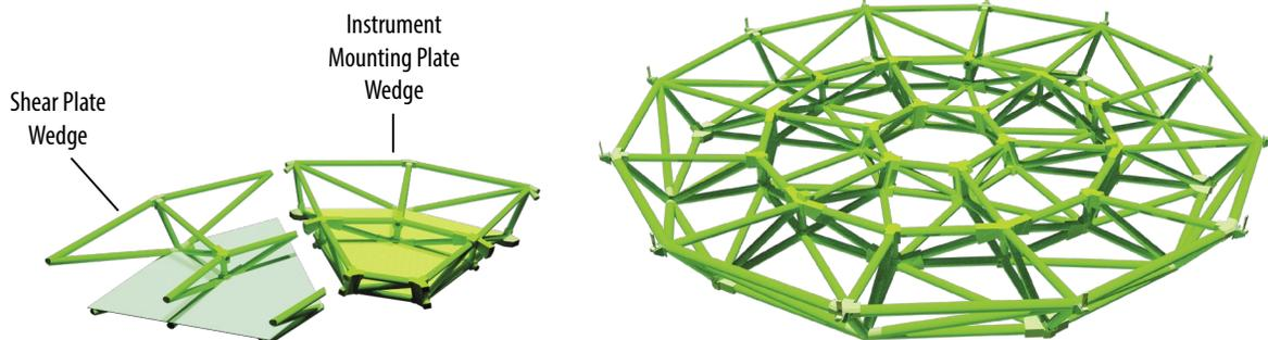
**Figure 2-29:** To optimize weight and strength, the PMBSS is a trussed design. The PMBSS is entirely beryllium to match the Coefficient of Thermal Expansion (CTE) of the Primary Mirror Segment Assembly. Three sets of PMBSS Wedge Subassemblies are fabricated and fastened together to comprise the whole PMBSS.
