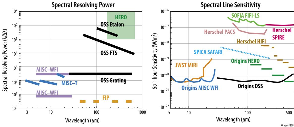
**Figure D-3:** *Origins* upscope option ideally complements the *Origins* baseline configuration by adding the capability of very high spectral resolution observations at high line sensitivity (HERO), by adding an mid-IR MISC imager , adding the 100 and 250 micron windows of FIPS and by increasing the mapping speed of OSS.
