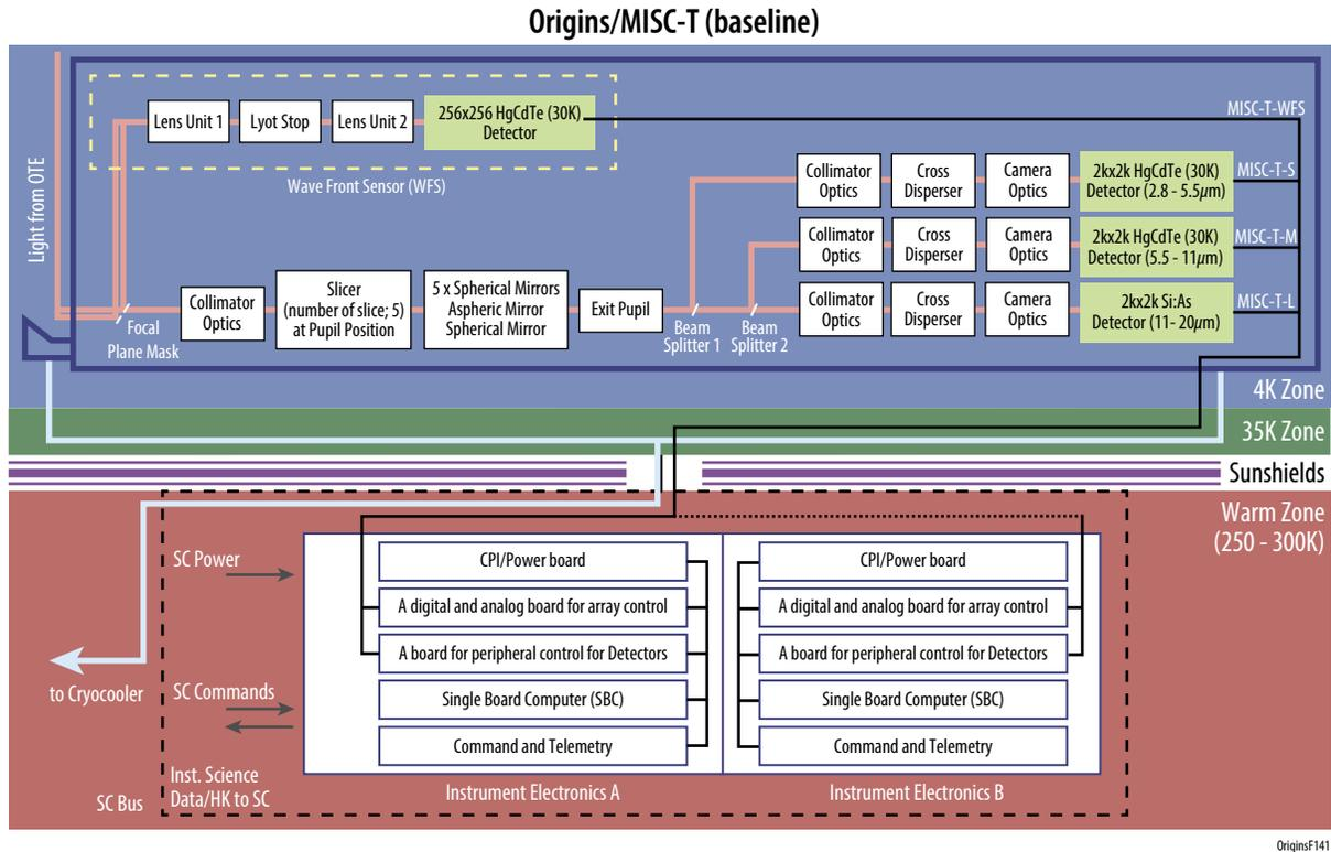
**Figure 3-14:** The MISC-T block diagram showing the optical paths, detector focal planes, electronics, and temperature regimes.
