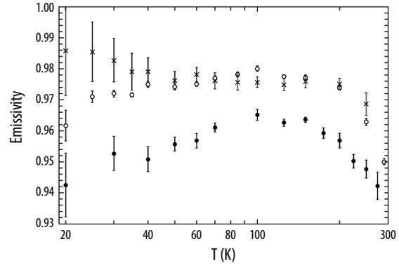
**Figure C-4:** Emissivity measurements made for BIRB show it is very black at low temperatures. The 0.65 kg/m<sup>2</sup> sample (X) used for JWST was also used in this model. This application of BIRB will be used for *Origins*.
