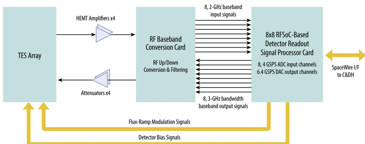
**Figure 3-28:** Detector readout scheme for FIP: FIP and RFSoc samples and processes signals simultaneously.
