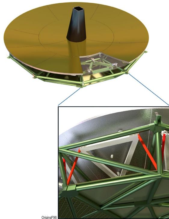
**Figure 2-28:** The Primary Mirror Segment Assembly Interface support structure recesses into the PMBSS truss elements and is supported by brackets to the lower truss elements.
