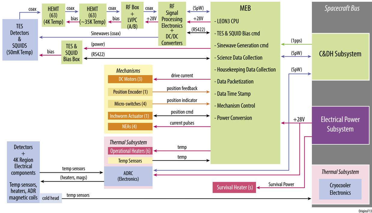
**Figure 3-8:** Block diagram of OSS instrument control. The mode complexity is comparable to instruments that have flown, such as *Herschel* SPIRE, and software re-use is estimated at 85%.
