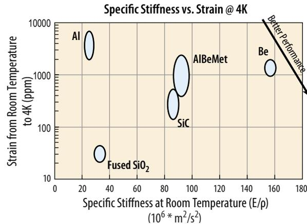
**Figure C-56:** Strain from room temperature down to 4 K against specific stiffness at room temperature shows tradeoffs between beryllium (Be), AlBeMet®, SiC and fused silica with aluminum (Al) as the lowest performer.
