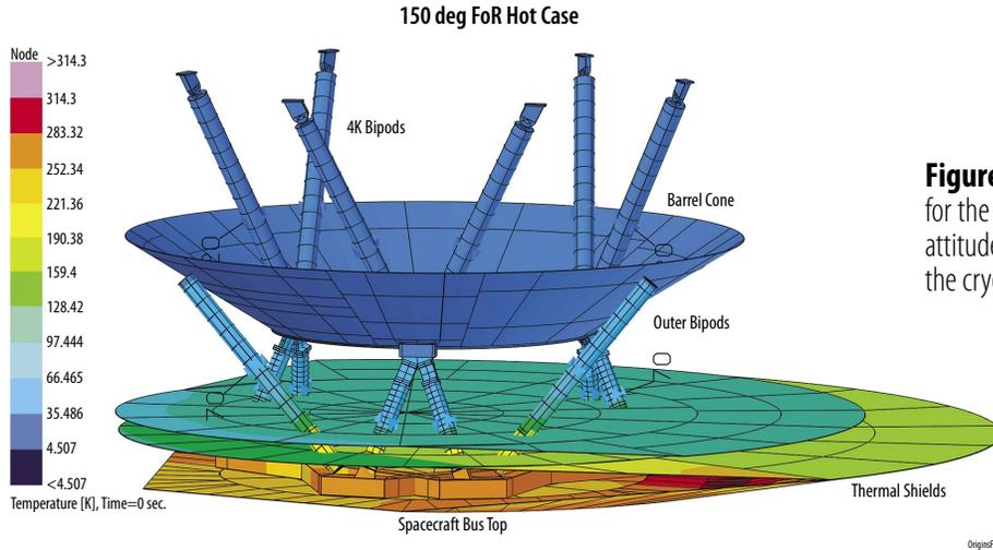
**Figure C-7:** The temperature contour plot for the Pitch +150° Hot case shows this EOL attitude produces the highest heat loads to the cryocoolers.
