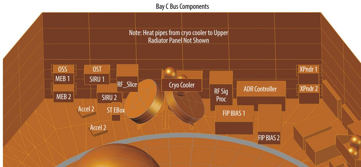
**Figure C-11:** There is plenty of space in each of the SBM bays for electrical boxes and other hardware. Here we show Bus Bay C.
