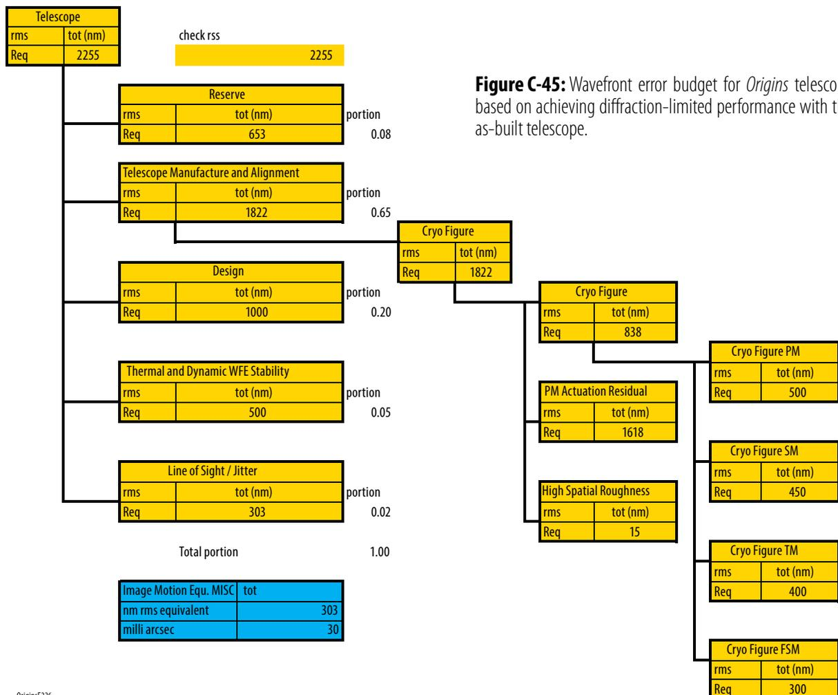
**Figure C-45:** Wavefront error budget for *Origins* telescope based on achieving diffraction-limited performance with the as-built telescope.
