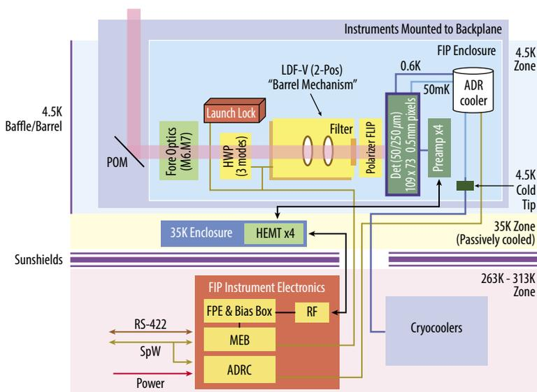
**Figure 3-25:** FIP has a simple design with one detector selectable by filter to 50 or 250  $\mu\text{m}$ . This Functional Block Diagram of FIP shows how the power dissipation in the cold 4.5 K section is minimized by placing the readout electronics in the warm part of the observatory.
