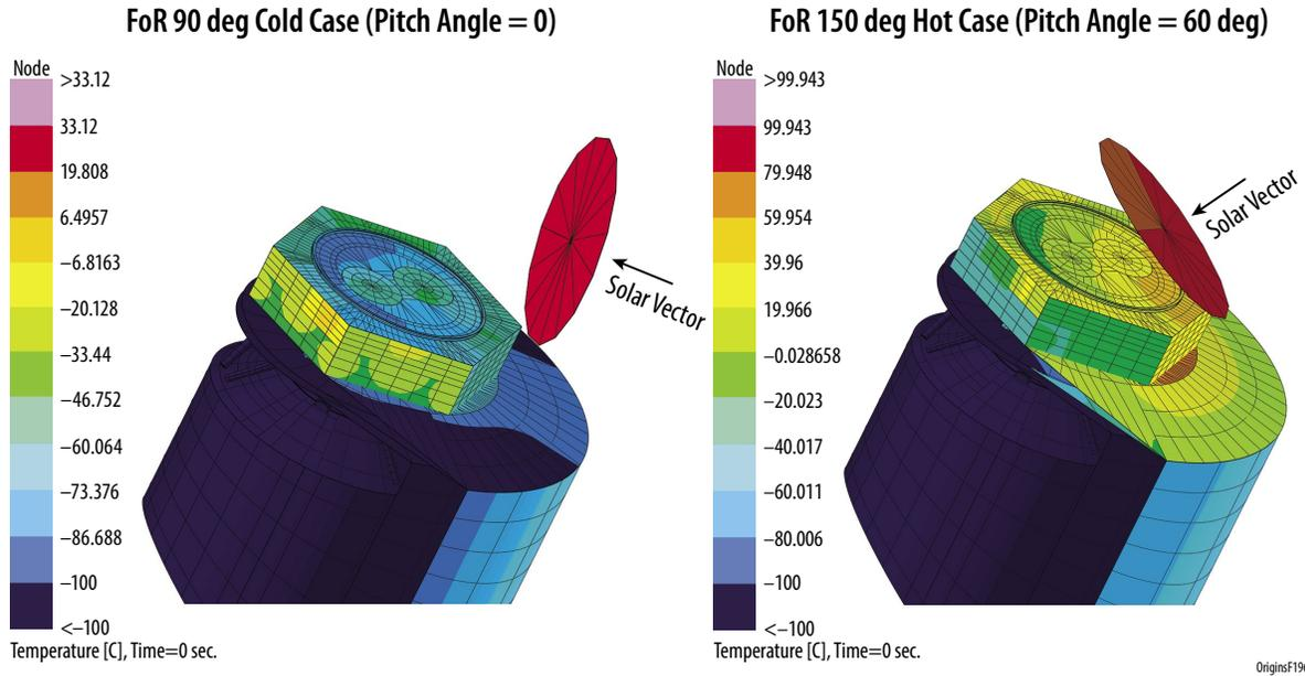
**Figure C-15:** The external surfaces of the outer Sunshield layer and SBM are all within the required bounds.
