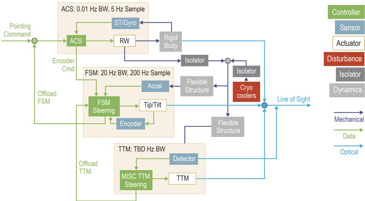
**Figure 2-33:** The *Origins* ACS multi-stage control loop architecture provides fine pointing accuracy and stability by actively suppressing the response of the telescope and instruments to internal disturbances.
