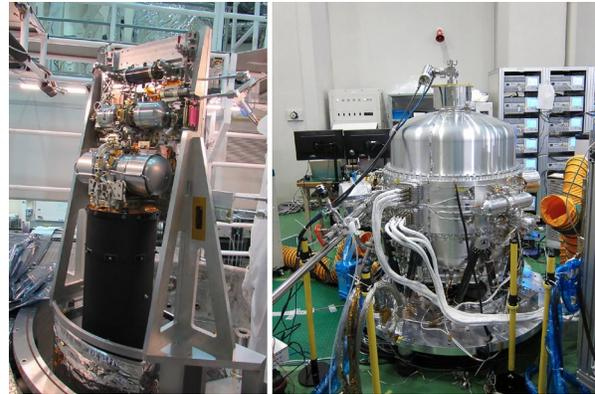
**Figure 2-6:** *Origins* baselines a cryocooler design adapted from present flight-worthy cryocoolers. Two examples of such are the MIRI cryocooler (shown in a test stand at left), or the several JAXA cryocoolers mounted on the Hitomi dewar (right).
