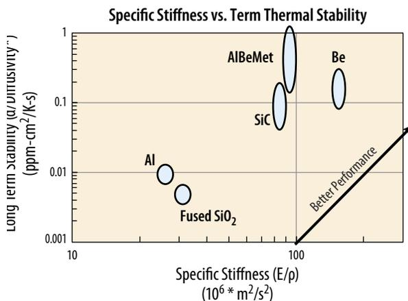
**Figure C-55:** Long-term stability (thermal diffusivity/CTE) plotted against specific stiffness at room temperature shows beryllium (Be), AlBeMet®, and SiC as the best performers.
