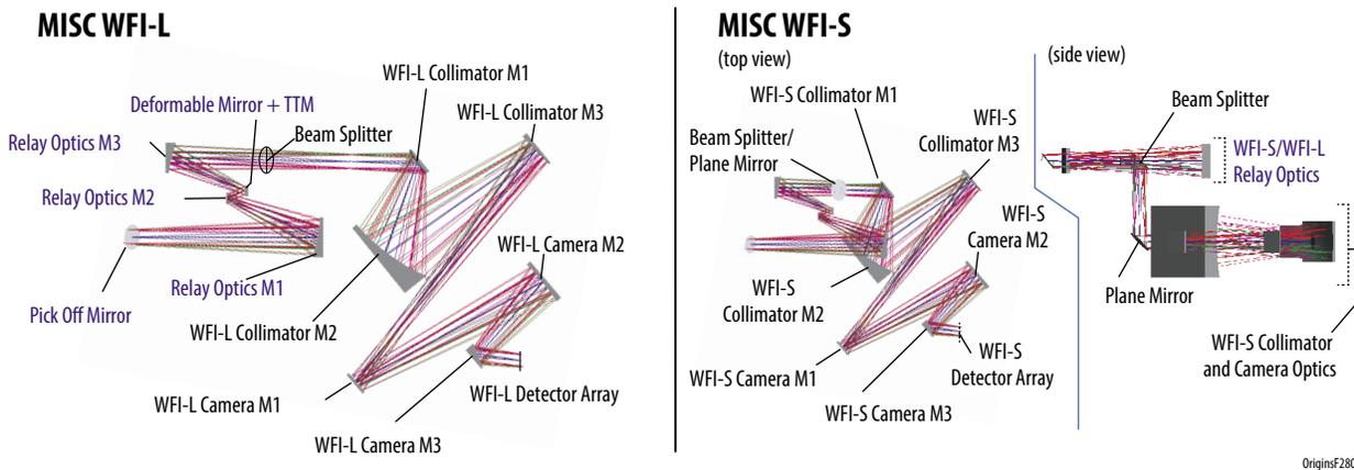
**Figure D-17:** The MISC WFI optical design includes a A) wave front error correction system in the fore optics and B) the imager optics.
