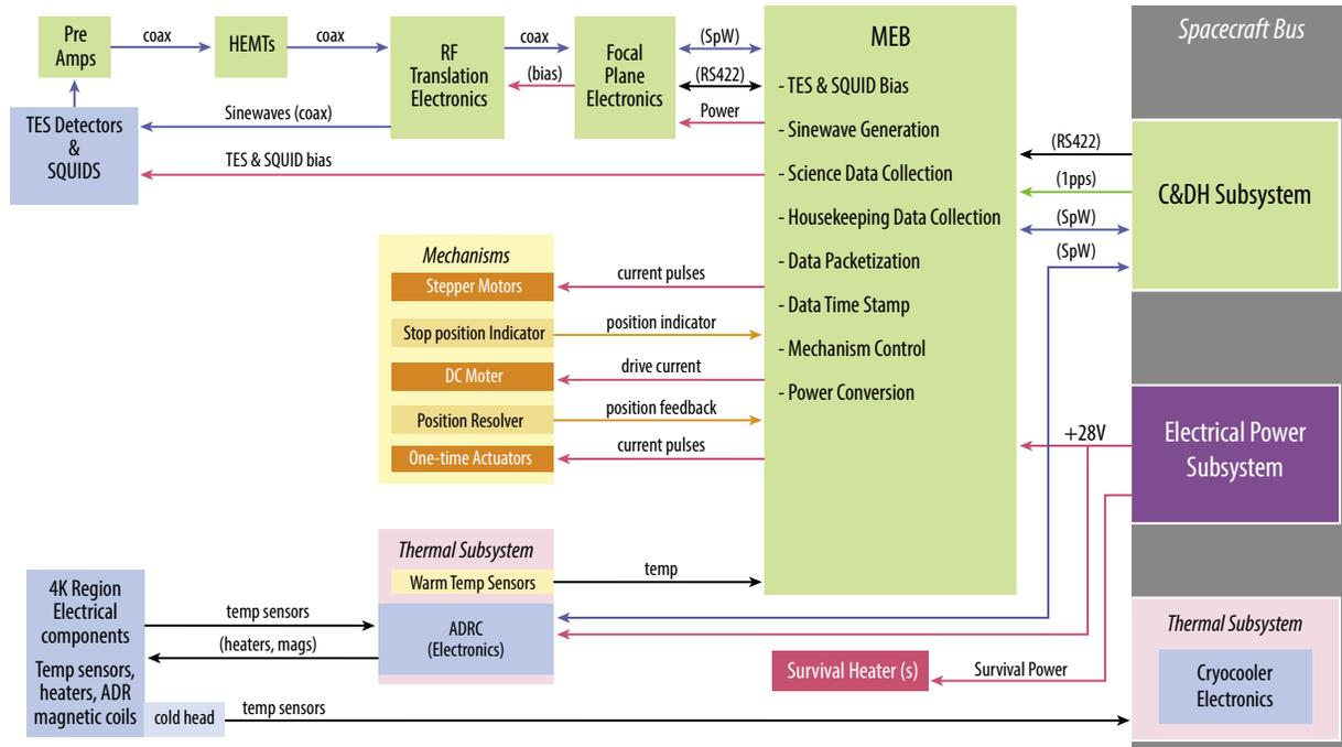
**Figure 3-31:** This FIP Block diagram shows how the instrument is controlled.
