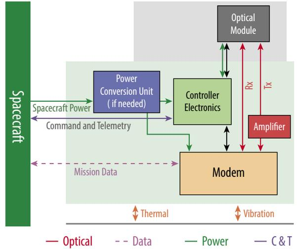
**Figure C-60:** Flight Optical Terminal Block Diagram
