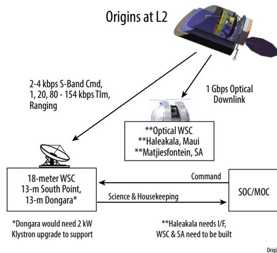
**Figure 2-38:** *Origins* Communication System Consists of Optical Downlink of Science Data and S-Band for Command & Telemetry
