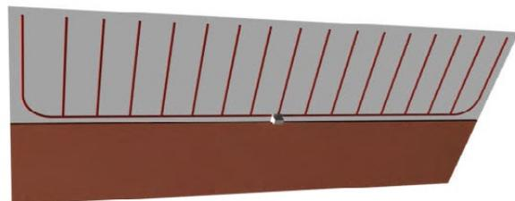
**Figure C-26:** The Spacecraft Bus Side Panel Radiators are split lengthwise to create two separate radiators – the lower acts as a heat sink for electronics and the upper as a radiator for cryocooler heat. The upper section has embedded heat pipes that transfer the heat from the cryocooler.
