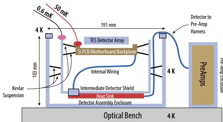
**Figure 3-30:** The FIP Focal Plane Array is cooled to 0.05 K and suspended within a 0.7 K enclosure, providing thermal shielding from the 4.5K stage. The Kevlar suspension, which is common to most instruments with low temperature detectors, provides for excellent stiffness while having a very low heat conductivity.
