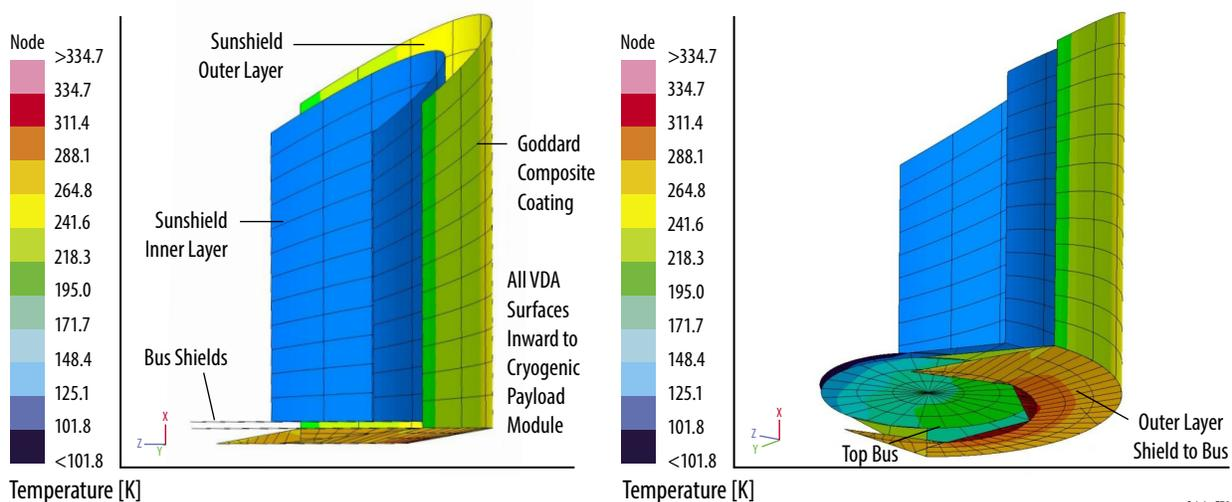
**Figure 2-11:** The Outer Sunshield with GCC maintains room temperature or lower for all FoR over nearly all of its surface.
