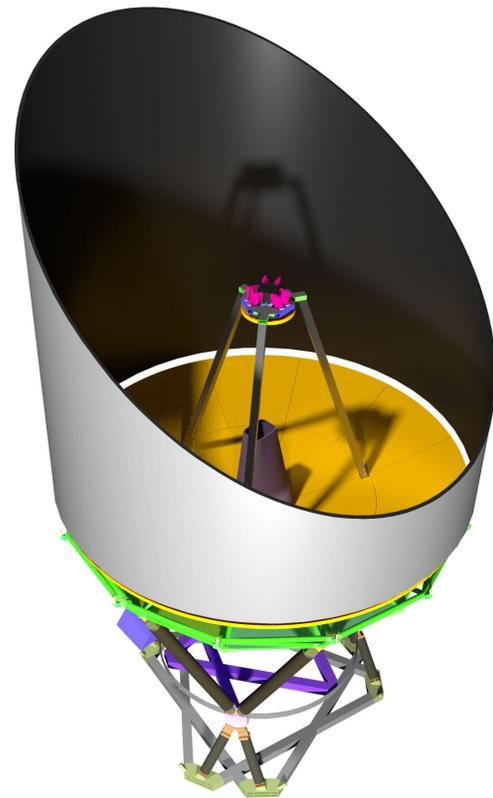
**Figure 2-16:** 4.5 K Baffle is supported from the PMBSS.
