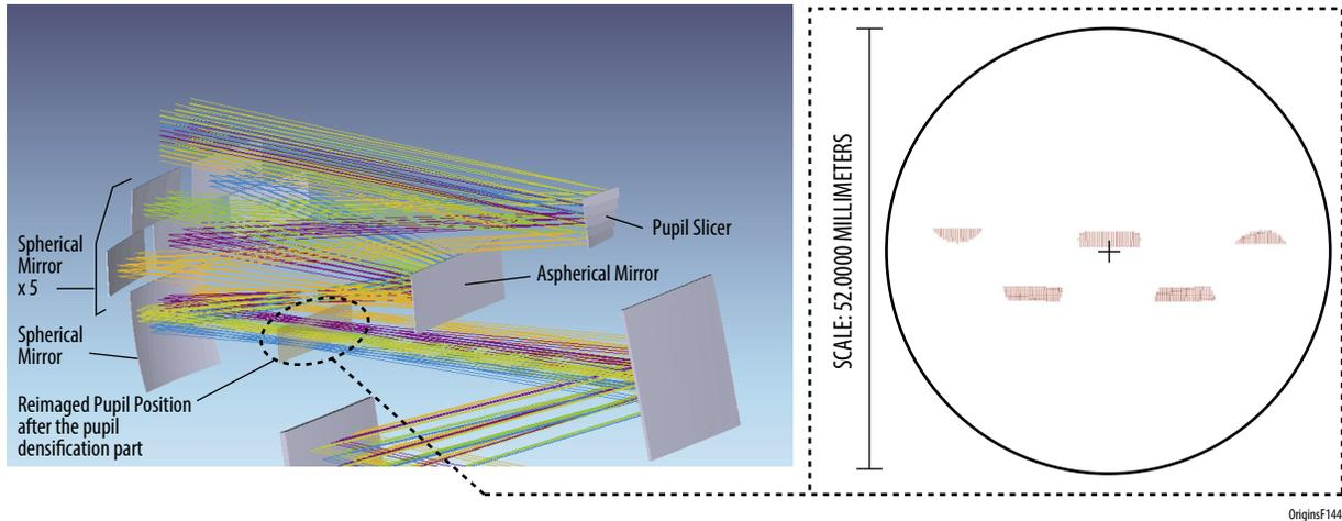
**Figure 3-17:** The telescope pupil is reimaged and sliced as shown at left, with the slices separated as shown in the image on the right.
