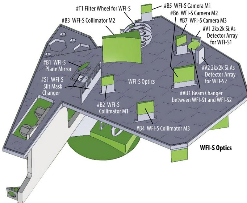
**Figure D-18:** The MISC WFI 3D solid model shows the instrument's A) WFI Fore optics, WFI-L optics, and B) WFI-S optics.
