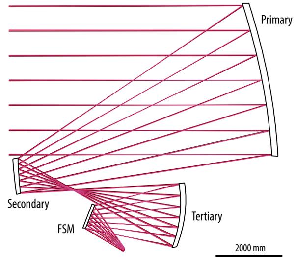
**Figure C-52:** Resulting optical design utilizing a spherical primary mirror. The design concept was not further pursued for *Origins* due to poor optical performance.
