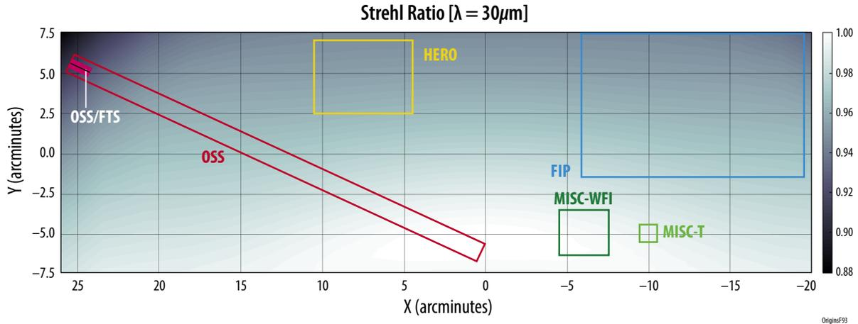
**Figure D-2:** An evaluation of the upscoped *Origins*' RMS wavefront error as a function of FOV shows that the performance requirement (less than  $0.07\lambda$ ) is met across each instruments FOV. Note that the colorbar is set such that light corresponds to better optical performance and dark to poorer optical performance.
