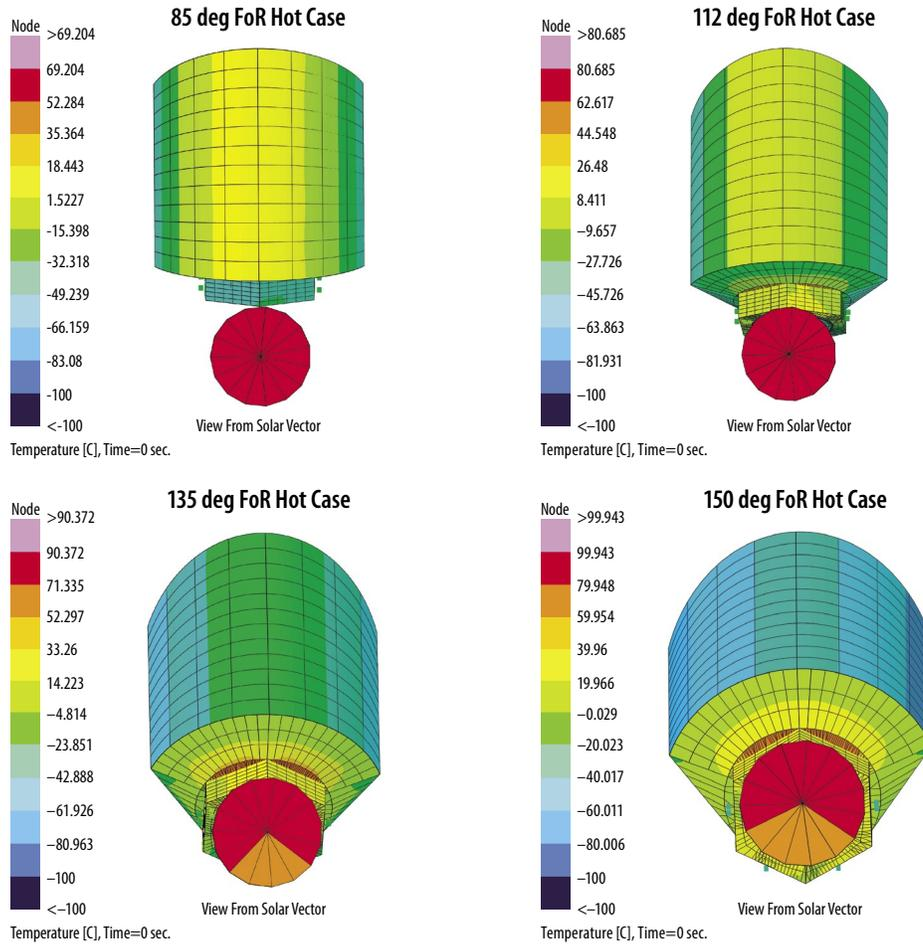
**Figure C-8:** Origins pitch angles of 85, 112, 135, and 150 degree (as viewed from the solar vector) shows the full FoR range accommodated by the thermal design. The inner shield and barrel are not visible in these views.
