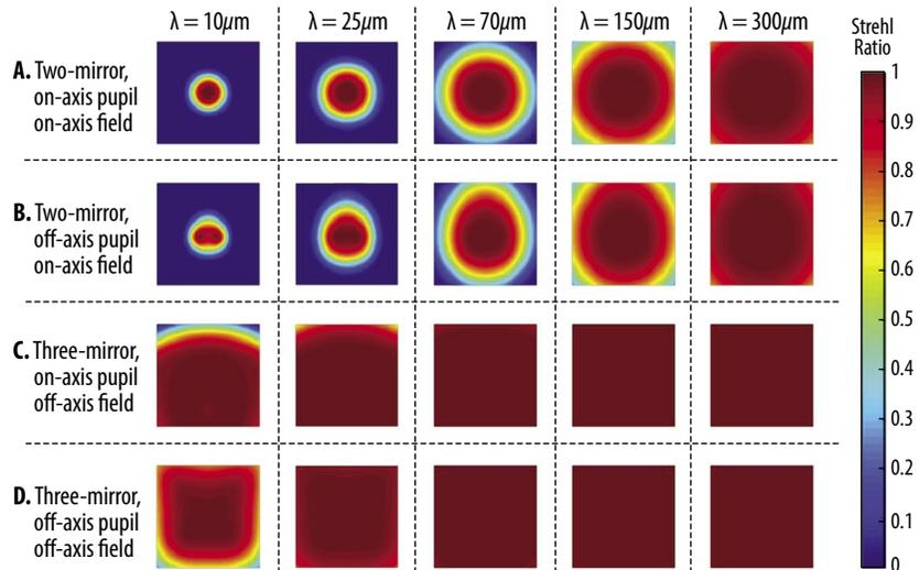
**Figure C-48:** Comparison of Strehl ratio as a function of FOV for four different telescope configurations. In each case the performance is evaluated over the same  $1^\circ \times 1^\circ$  full FOV.
