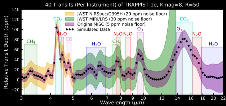
Origins' mid-IR spectrometer, MISC, is designed with the wavelength coverage and precision necessary to detect biosignatures (O<sub>3</sub>+N<sub>2</sub>O, O<sub>3</sub>+CH<sub>4</sub>) in nearby terrestrial exoplanets. JWST's anticipated noise floor is significantly higher, and will require twice as many transits, than Origins'.
