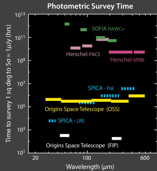
The Origins Space Telescope will map wide fields of view orders of magnitude faster than previous and planned missions, with instruments that provide low (FIP) or moderate spectral resolution (OSS).
